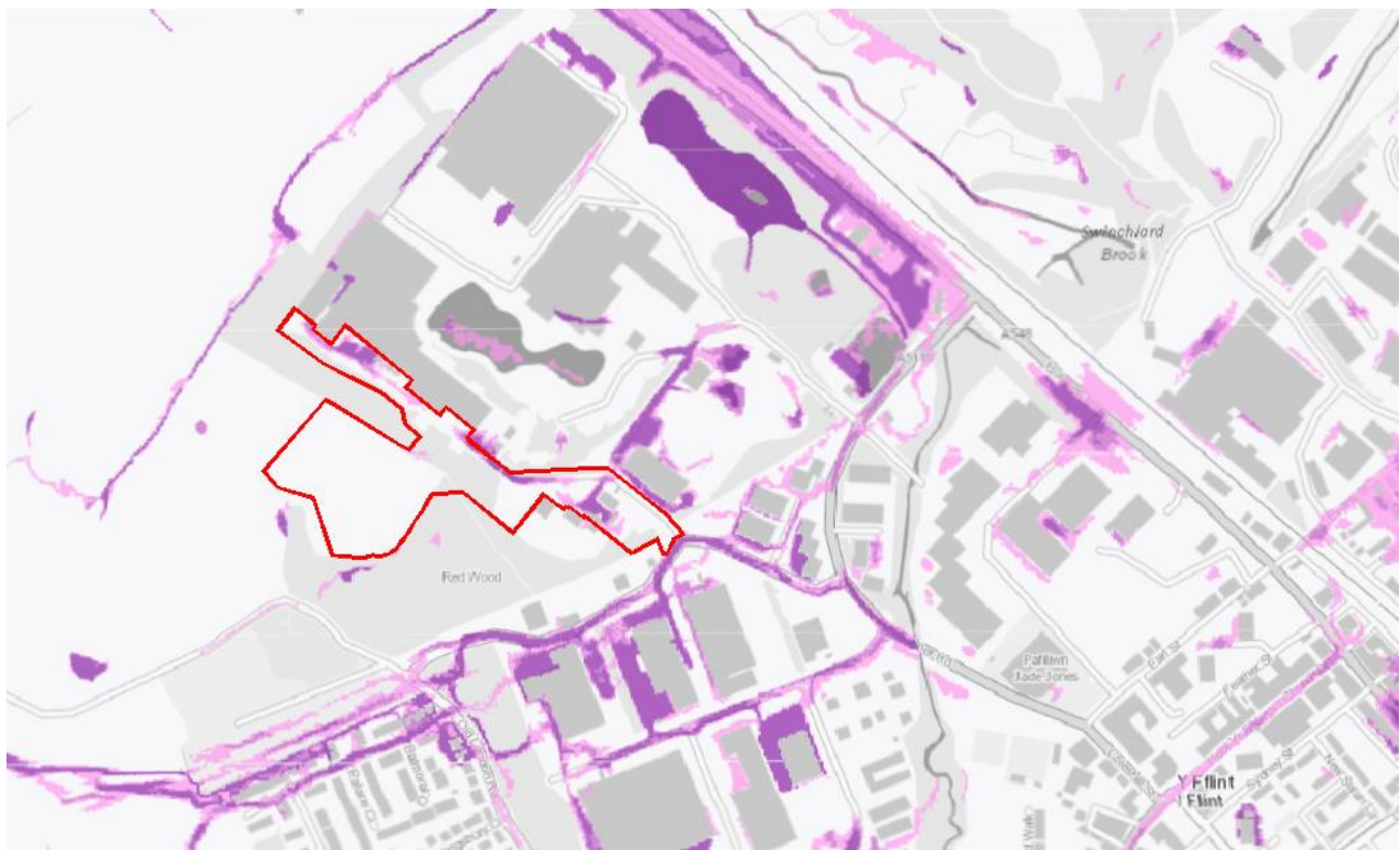
Figure 4 - Excerpt from NRW surface water flood risk map, with proposed site boundary overlaid.
