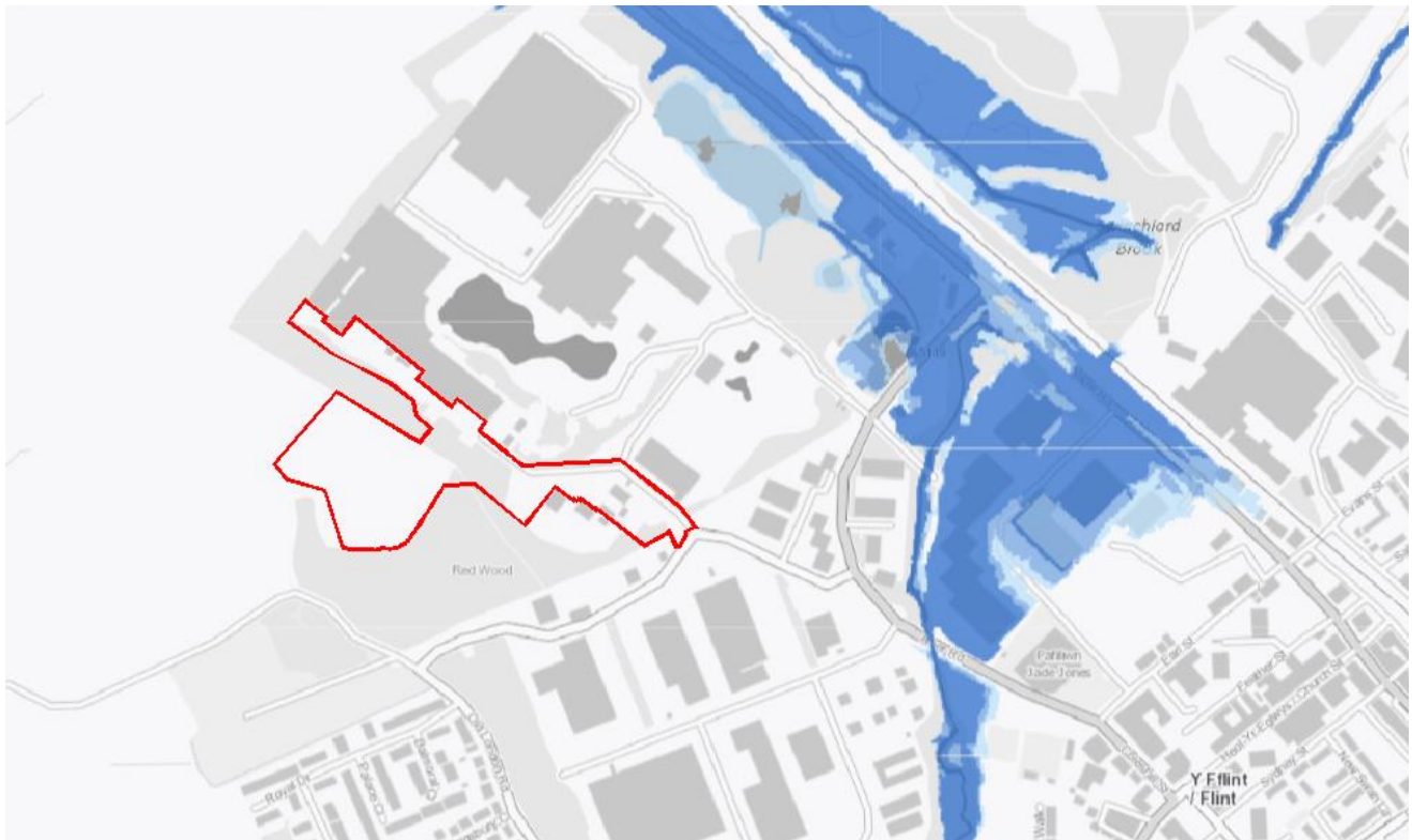
Figure 2 - Excerpt from NRW fluvial flood risk map, with proposed site boundary overlaid.
